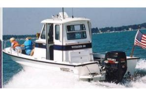
LOA: 23'-3" • BEAM: 8'-6" • DRAFT (hull): 14" • WEIGHT (no engine): 3000lbs MIN HP: 115 • MAX HP: 250 • COCKPIT DEPTH: 22" • TRANSOM HEIGHT: 25" FUEL CAPACITY: 73gal • RANGE (225hp, 90%): 230mi • SPEED (225hp): 41mph
