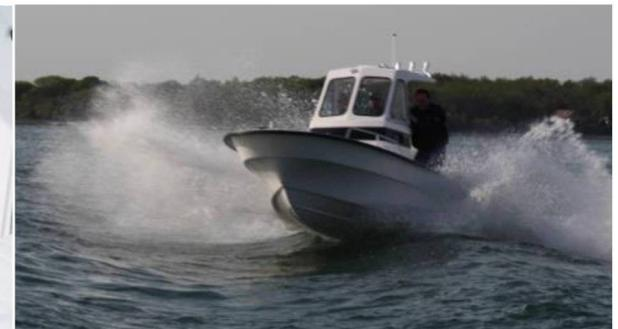
LOA: 20'-9" • BEAM: 7'-7" • DRAFT (hull): 12" • WEIGHT (no engine): 2100lbs
